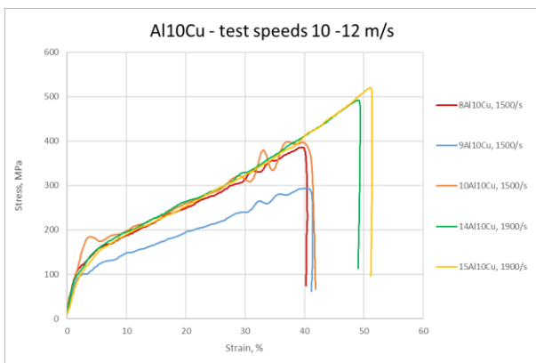
Fig. 2 SHPB dynamic test results at 10-12 m/s
