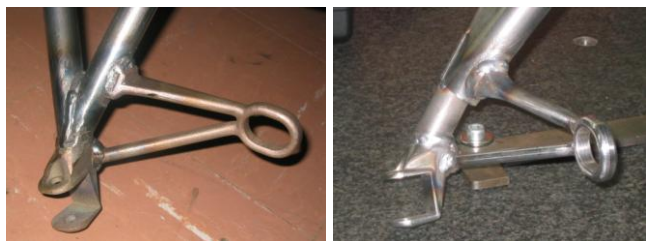
Fig. 1 Result of Rapid Prototyping for learning and communication purpose. Exhaust and foot holder BMW motorcycle component made with DMLS (left side) and with CNC rapid prototyping technology (right side of Fig.) [1]
