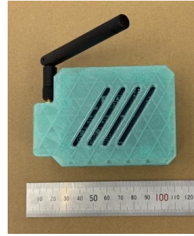
Fig. 8 IoT device built on Arduino with a Sigfox module in a 3D printed case (width 95 x height 65 x depth 40 = volume 247,000 mm 3 )
