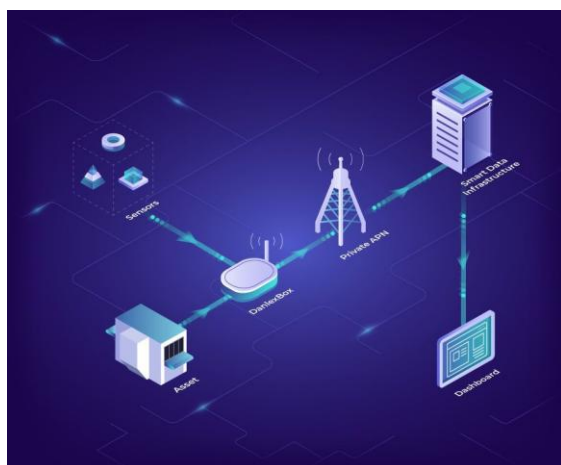
Fig. 3 Connectivity to the PM4X Infrastructure
