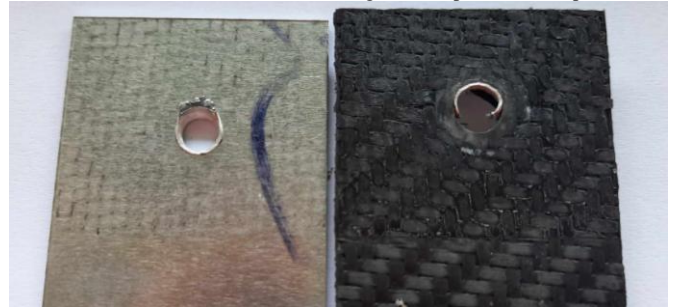
b) Al-CF RD, partial shear of the bushing (approx. 2/3 of the circumference), the bushing remains wedged in the CF
