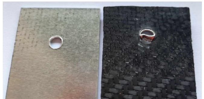
c) Al-CF RD, total shear of the bushing, the bushing remains wedged in the CF
