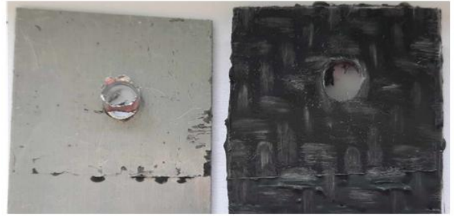
a) Al-GF RD, partial shear of the bushing (approx. 1/3 of the circumference), the bushing remains part of the Al plate
