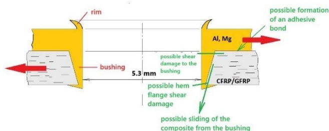
Fig. 1 Schematic representation of a possible joint failure
