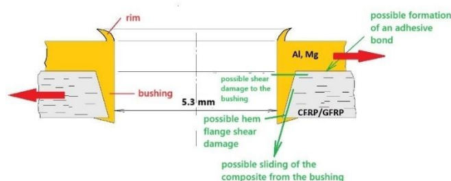
Fig. 1 Schematic representation of a possible joint failure
