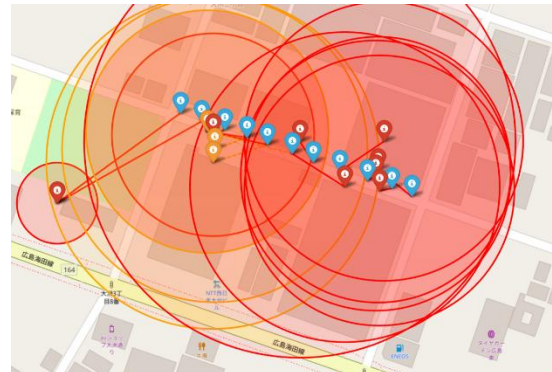
Fig. 9 Plot of actual coordinates and positioning results in the 110-m section (single vs. continuous).
