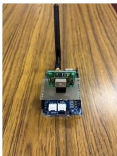
Fig. 1 IoT device with Sigfox network and GPS modules.
