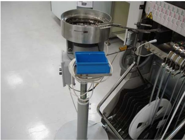
**Fig.8.** Vibrobunker system
