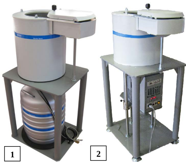
Fig.1. Laboratory HPGe gamma-spectrometer with shield: 1 - with liquid nitrogen cooling and 2 - with cooling system based on Stirling electrical cooler LSF9340-02 (Thales, France).
