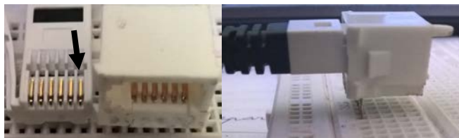
Fig. 1 BTA male and female connectors (from left side). First pin of the male BTA connector is marked with black arrow.
