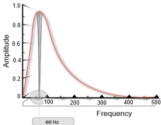
Fig. 5. Schematic representation of a typical EMG power spectrum [10]
