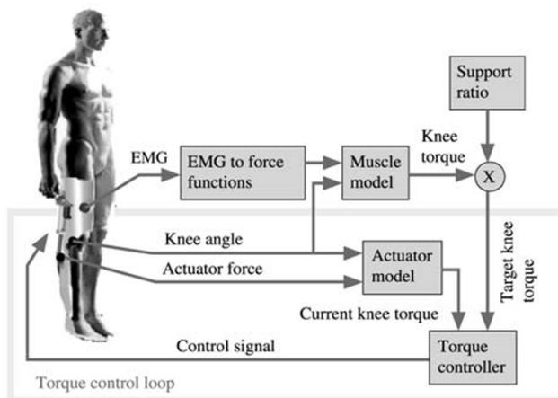
Fig. 9. Orthosis with the direct force control system [13]
