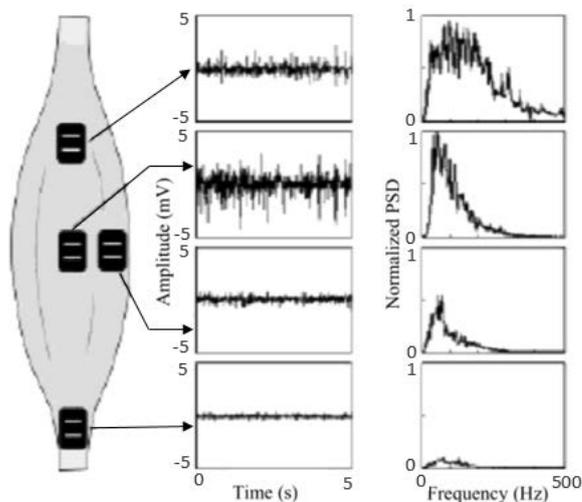
Fig. 6. Signal amplitude dependence on electrode location [9]
