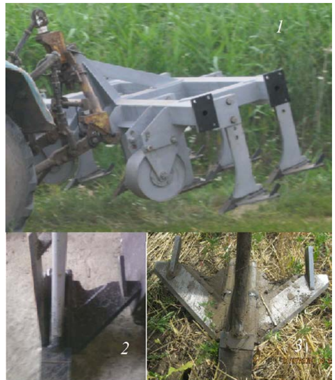
Figure 1 – Chisel plow with options of a working element 1 – the chisel plow of the new generation; 2 – position "flat cutter"; 3 – position "chisel".
