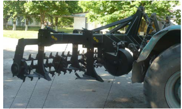
Figure 2 – Chisel plow with a roller: 1 – frame; 2 – supporting wheel; 3 – working element; 4 – roller-ripper
