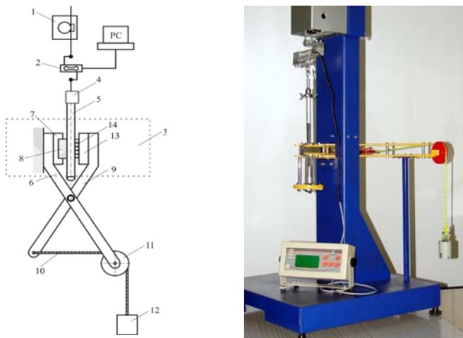
**Fig. 2.** The scheme and the laboratory test machine to measure coefficient of friction on specifically length with one-sided sliding
