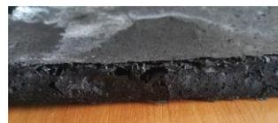
Fig. 5. Defective PVC board
