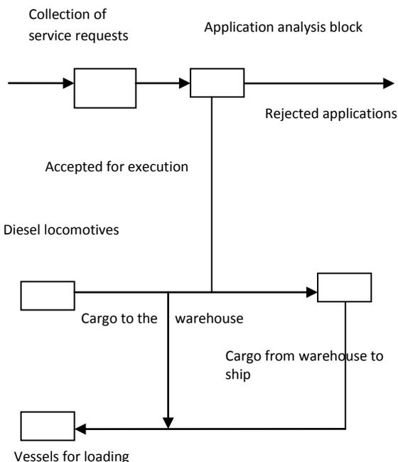
Fig. 1. The block diagram of cargo handling technological processes at the port
