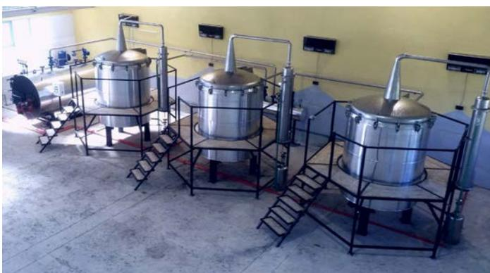
Fig. 6 Complete equipment for essential oil distillation with new solution of the substance flow system (produced by "Solar mont" Ltd, Gradiska, B&H)
