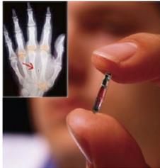
Radio-frequency identification chips (RFID), compatible with human tissue, are implanted in the human body. The passive RFID chip could be inserted in the human hand and used as a unique human bar code. The size of the microchip and its antenna is just 11.1 x 2.1 mm. When the RFID chip is brought for a couple of seconds near a
