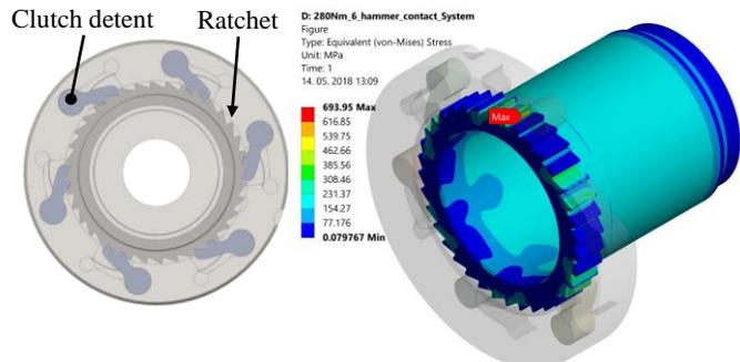
Figure 4. (a) Custom freewheel clutch solution as a cheaper and more reliable alternative to commercial sprag clutches; (b) evaluation of internal stresses due to pedalling torque transfer using FEA.
