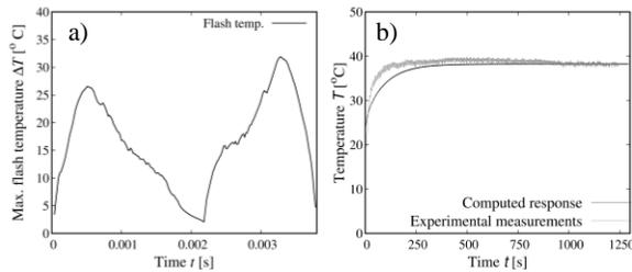
Figure 2. Evaluation of the flash (a) and nominal (b) temperature rise due to frictional effects during gear meshing (example results for POM-PA66 gear pair with 1Nm torque load and 1392rpm)
