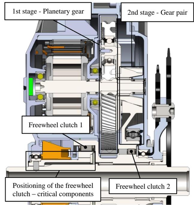
Figure 1. Pedelec drive train solution
