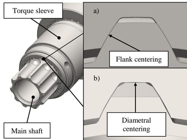
Figure 3. Torque sleeve and main shaft spline joint: (a) flank positioning- insufficient positioning accuracy; (b) outer diameter positioning – adequate centering of the sleeve
