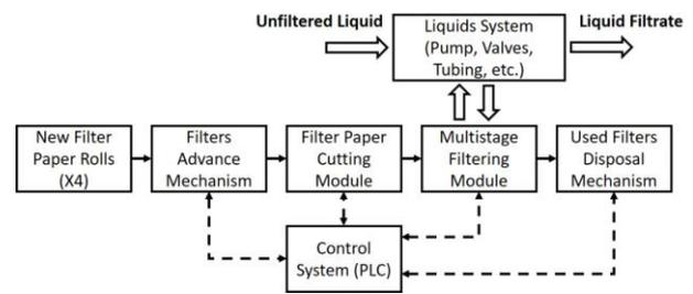
Fig. 2 Structure of the designed automatic filtering system.
