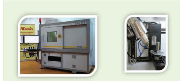
Photo 13 X-ray computer tomography, type Nikon XT H 225
