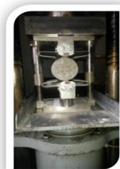
Photo 10 Splitting tensile strength
