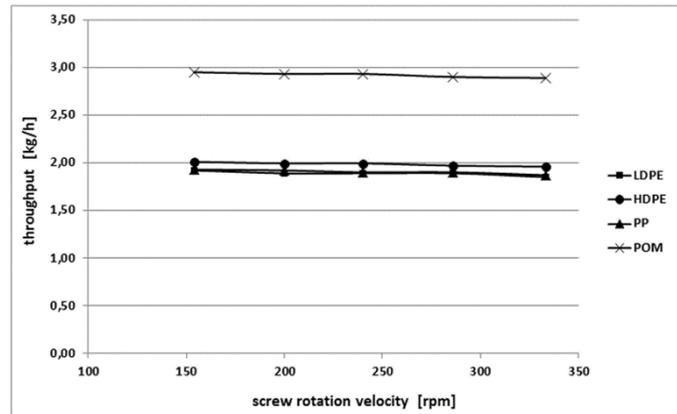
Fig. 13 Throughput of the injection process at variable screw rotation velocity
