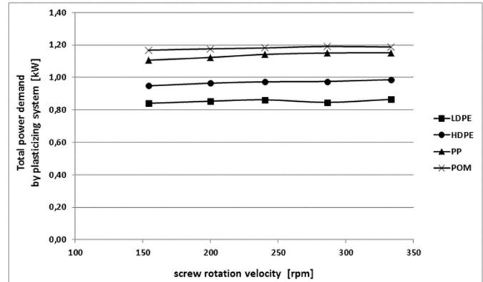
Fig. 12 Total power demand by plasticizing system at variable screw rotation velocity
