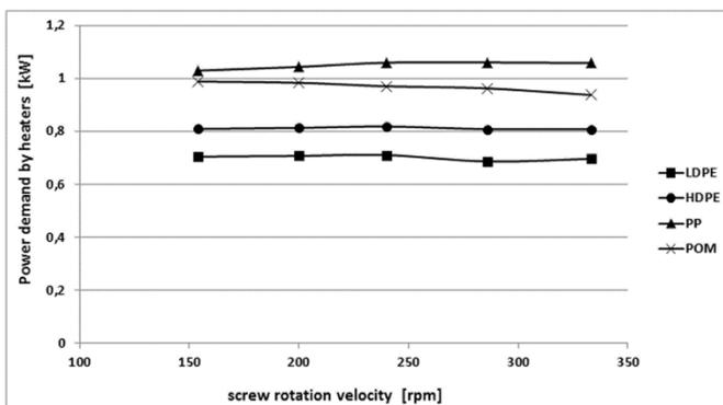
Fig. 10 Power demand by heaters at variable screw rotation velocity
