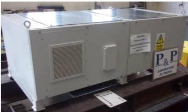
Fig. 7. Full-scale power converter during vibration testing
