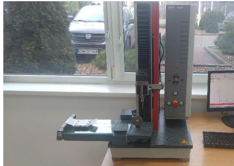
2.1.1. The machine Zwick / Roell testing machine equipped with appropriate fixturing to determine the coefficients of friction. The equipment used to measure the COF of the film.
