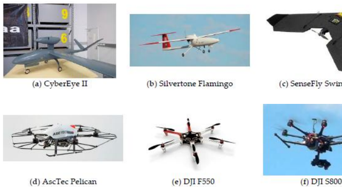
Figure 1: Example of a small fixed wing (a) CyberEye II; (b) Silvertone Flamingo; (c) SenseFly Swinlet and rotary wing (d) AscTec Pelican; (e) DJI F550; (f) DJI S800 unmanned aircraft (All the UAVs shown are part of the fleet of the Australian Research Centre for Aerospace Automation).
