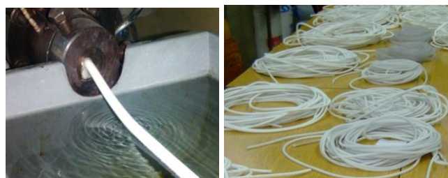
Fig. 1 View of the extruded rod and fragments of the produced samples.
