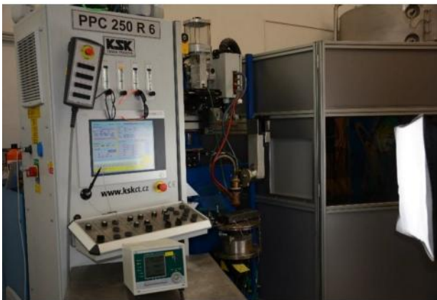
Fig. 1 The plasma hardfacing machine PPC 250 R6 with plasma transferred arc (PTA) technology.
