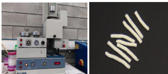
Fig. 4 View of MFI instrument, Ceast 6542.0 and selected measurement samples
