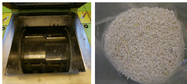
Fig. 2 Appearance of the shredder knives and PVC recycle.
