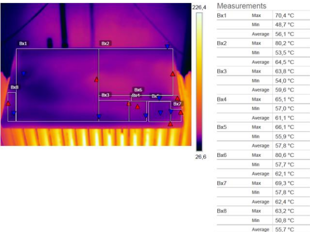
Fig. 3. Temperature distribution on the wall of the beehive after the 14th minute of the experiment.
