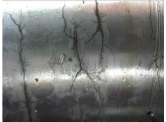
Fig. 1: The surface of the worn-out roll \varnothing 300 mm
