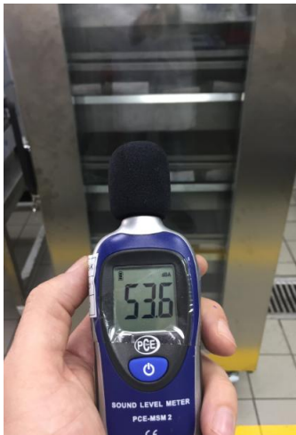
Fig. 8 The noise level measurement value of the innovative blood storage refrigerator prototype.
