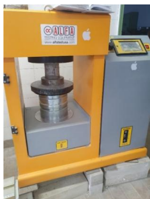
Photo 8 Concrete compressive test
