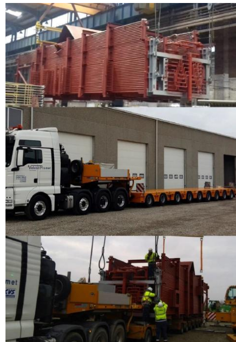
Fig. 1 Steam boiler module transport
