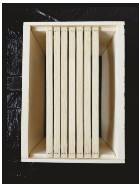
Fig. 1. Prototype of an innovative collapsible beehive made of quartz ceramic items with assembly profiles.
