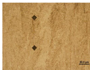
Fig. 7 Microstructure of fist cladded layer with Dievar
