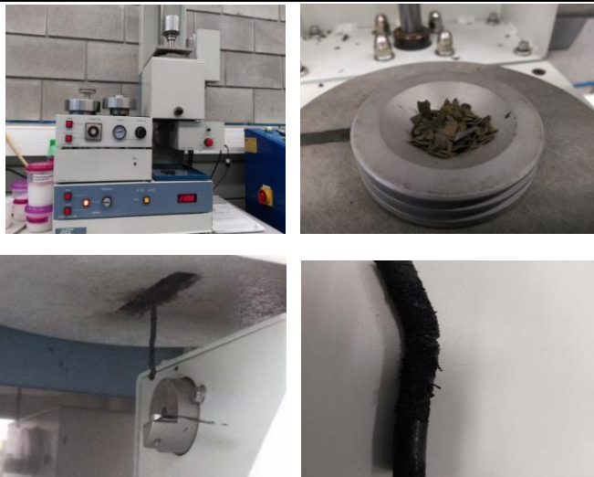
Fig. 6 View of MFI instrument, Ceast 6542.0 and selected measurement samples.
