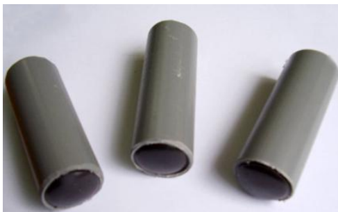
Fig. 2 Cartridges charged with non-detonating chemical mixture [2,6]
