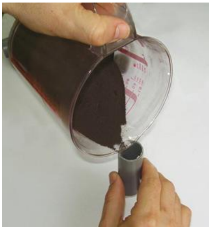
Fig. 1 Charging the cartridges with non-detonating chemical mixture [2,6]
