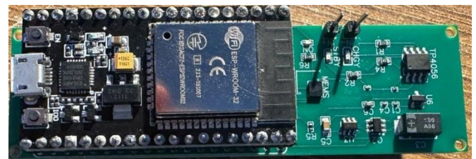
Fig. 1 Prototype of MEMS-based sensor which could be use in WSN architecture.
