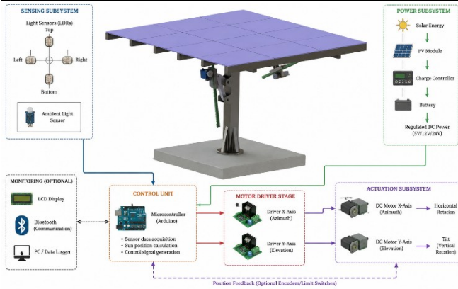
Fig. 2 Overall system architecture of the dual-axis solar tracker
