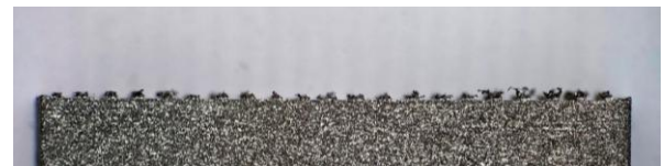
Fig. 4 Detailed view of burr formation at the groove edge
