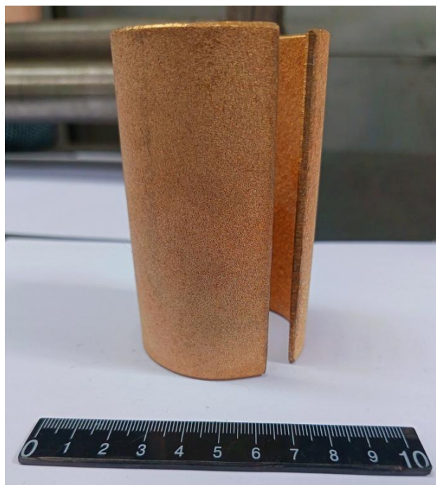
Fig. 2 A rolled tubular blank with a diameter of 60 mm.
