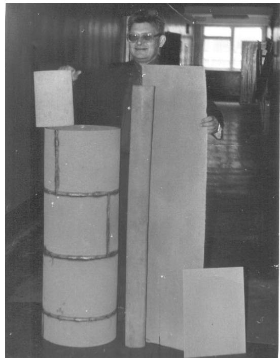
Fig. 5 Sintered sheet blanks and filter elements made on their basis by rolling.
