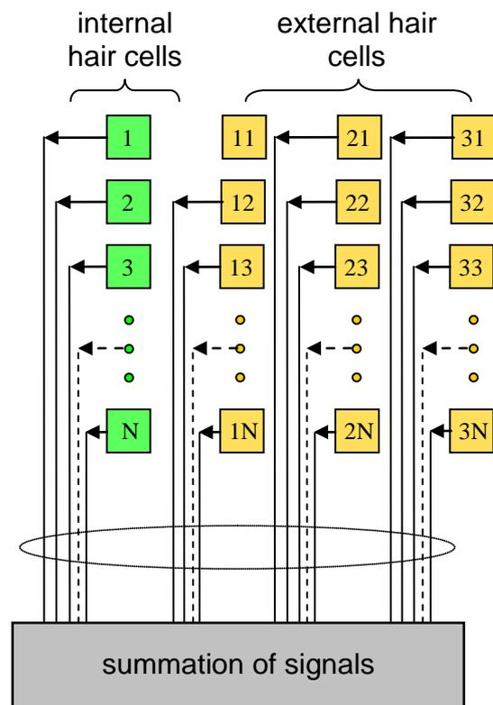
Fig. 1. Structure of the imitation model of the inner ear function
