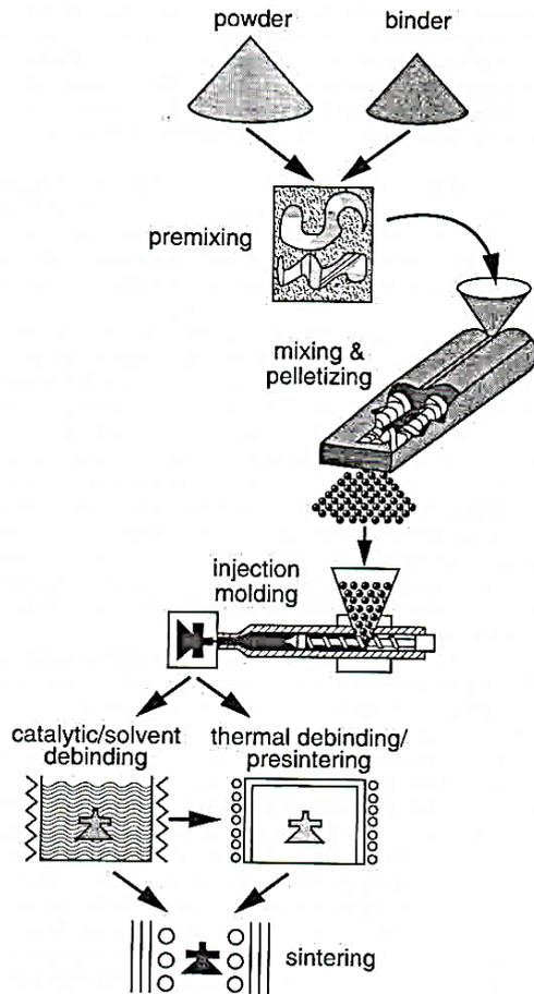
Figure 2 Flow chart of powder injection molding method [7]
