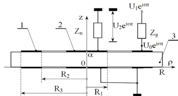
Fig. 1. Calculation scheme of disk piezoelectric transformer
