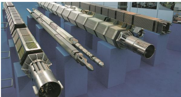
Figure 1 - Typical design of fuel assembly
