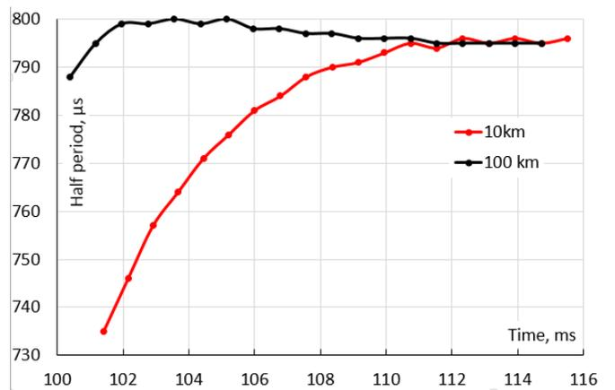
**Fig. 4** Dependence of the duration of half-periods of damped oscillations of the signal of the transient process on the time of its existence at different distances from the beginning of the line.
