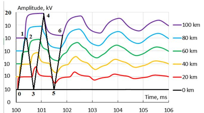
Fig. 2 Transient signals at different distances from the beginning of the line.
