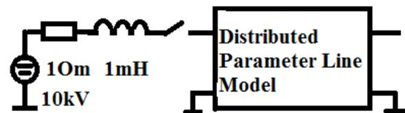
Fig. 1 Signal "Voltage step" generation circuit at the beginning of the line.
