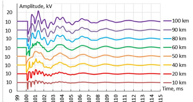
Fig. 8 Transient signals for "Soliton" generation circuit in the middle of the line.
