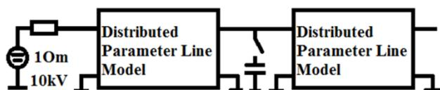
Fig. 7 Signal "Soliton" generation circuit in the middle of the line.
