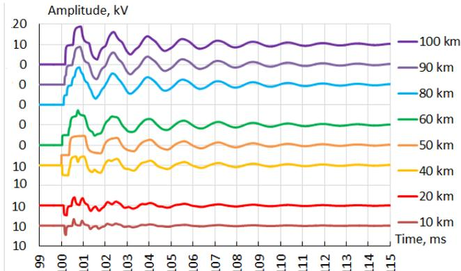
Fig. 5 Transient signals at different distances from the beginning of the line.
