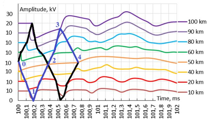
Fig. 9 The trajectory of a traveling wave at different distances from the beginning of the line.
