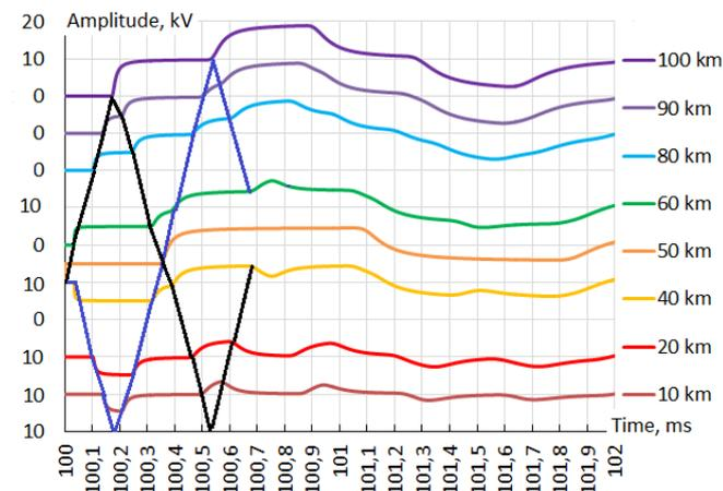
Fig. 6 The trajectory of a traveling wave at different distances from the beginning of the line.
