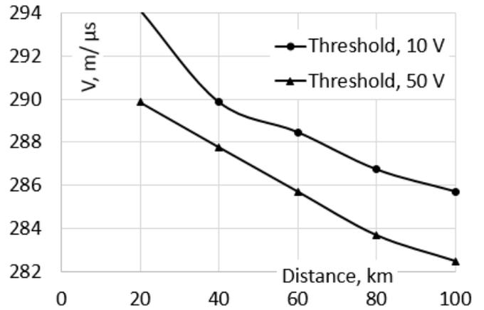
**Fig. 3** The recorded average velocity of propagation of the traveling voltage wave of the terrestrial mode at different distances from the beginning of the line.
