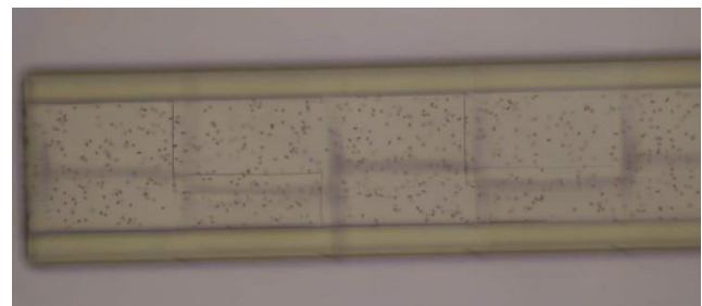
Fig. 13 Image of the developed hollow micro-channel filled with a diluted erythrocyte suspension
