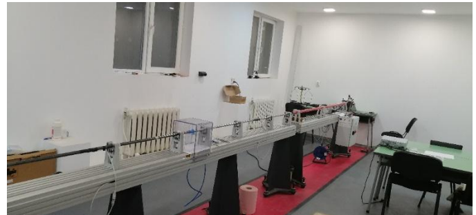
Fig. 1. A Split Hopkinson Pressure Bar system designed for testing of metals
