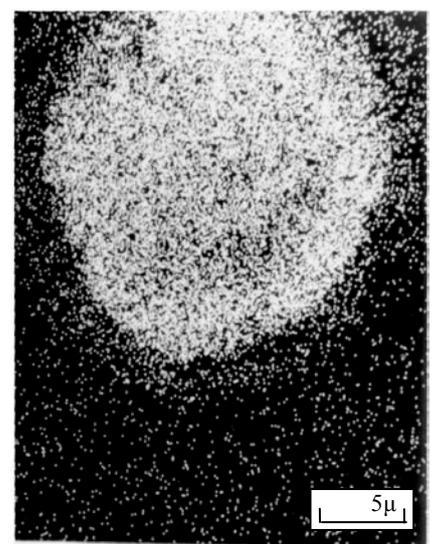
**Fig.4** Carbon migration from graphite and “halo” formation with increased carbon content B4500-2 upon electron beam treatment with  $E_s=2 \cdot 10^3 \text{ J/cm}^2$ .
