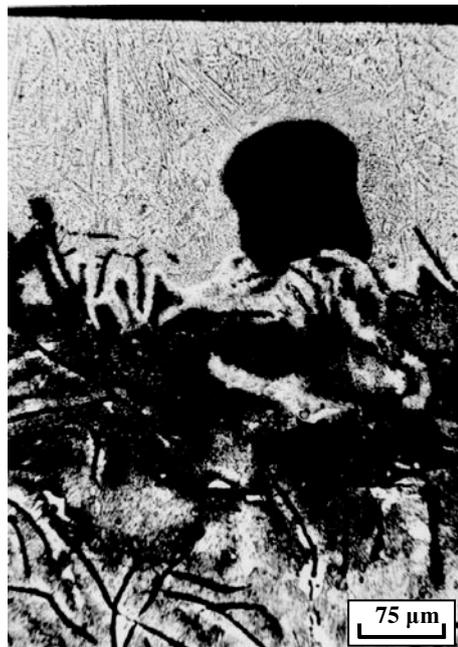
**Fig.2** Incompleteness due to partial evaporation of graphite inclusion at the bottom of the molten bath in GG 15 upon laser treatment with the following parameters:  $N_s=1.9 \cdot 10^4 \text{ w/cm}^2$ ,  $E_v=1.58 \cdot 10^4 \text{ J/cm}^3$ .
