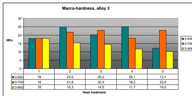
Figure 1÷3 Data for hardness of the alloys
