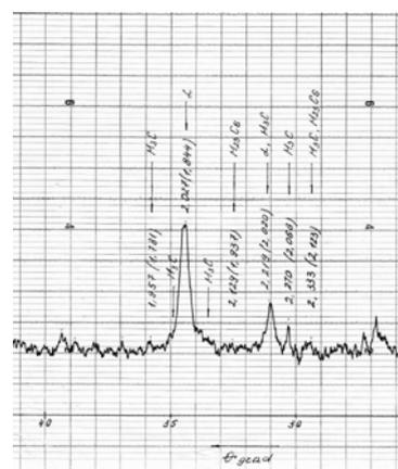
Figure 4. X-ray diffraction of the alloys after homogenization
