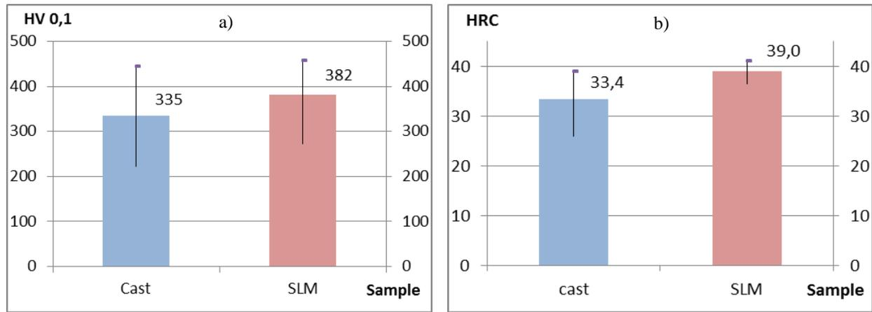
Fig. 7. Vickers hardness: a) and Rockwell hardness; b) of samples produced by casting and SLM.
