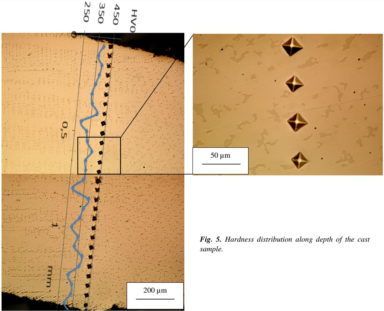
Fig. 5. Hardness distribution along depth of the cast sample.
