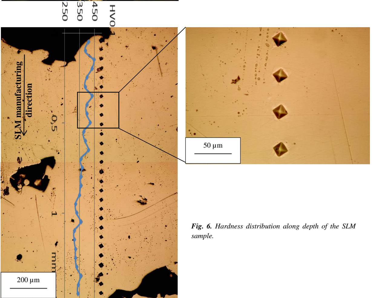
Fig. 6. Hardness distribution along depth of the SLM sample.
