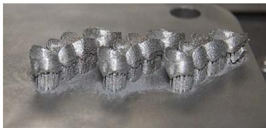
Fig. 1. SLM of dental bridges
