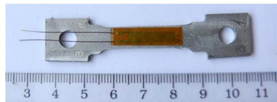
Fig. 4. SLM tensile test specimen with strain gauge.
