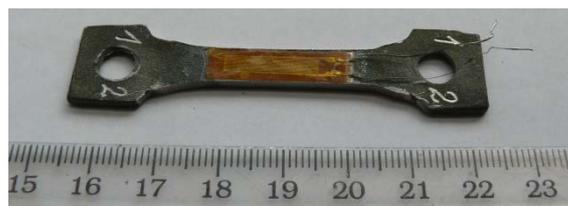
Fig. 3. Cast tensile test specimen with strain gauge.
