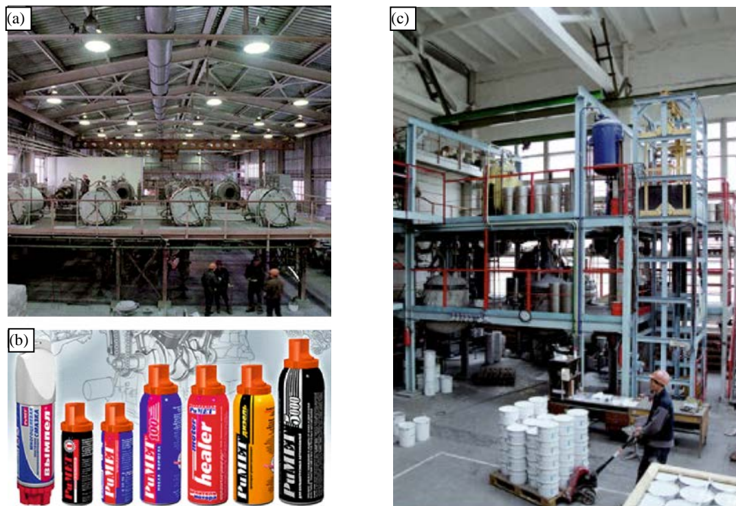
Fig. 32. Production of metal powder by gas-phase synthesis and powder-based materials at “Akademicheskii” Research and Development Center: (a) production of zinc powder; (b) products based on bronze powder for the protection of frictional surfaces; (c) production of zinc-enriched paint.
