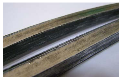
Fig. 2. CP Ti samples after SPD processing
