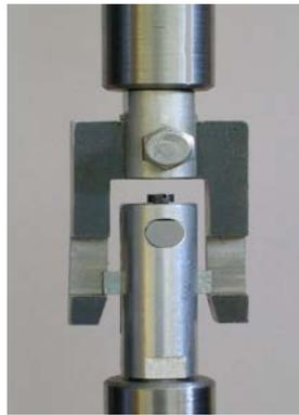
Fig. 4 Modified bending tests (notch toughness test).
