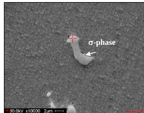
Fig. 7. Structure of \sigma -phase in the feather, SEM
