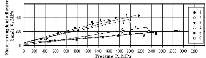
**Fig. 8.** Effect of pressure on the shear strength of adhesive bonds for samples with different microstructures: 1 - CG (without coating); 2 - UFG (without coverage); 3 - CG with TiC; 4 - UFG with TiC; 5 - CG with TiO<sub>2</sub>; 6 - UFG with TiO<sub>2</sub>.
