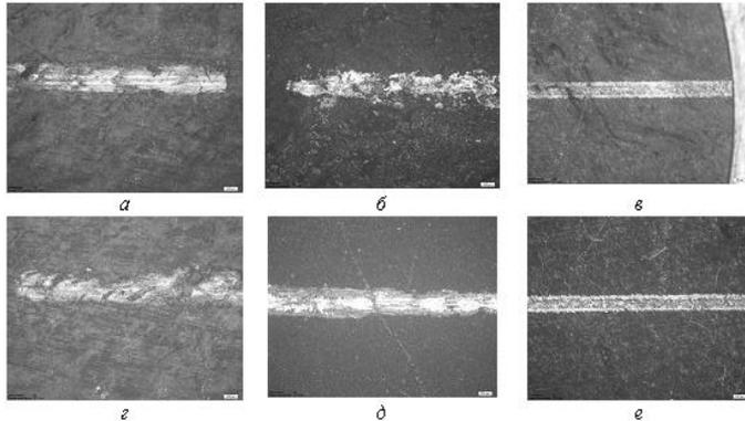
**Fig. 6.** Friction paths obtained during the tribological tests according to the scheme of linear reciprocating motion: a - commercially pure titanium Grade 4 without coating with a CG structure; b - commercially pure titanium Grade 4 with a CG structure with IPS coating (TiC); c - commercially pure titanium Grade 4 with a CG structure with a coating obtained by the MAO technology (TiO); d, e, f - the same with a UFG structure (3 times magnification).
