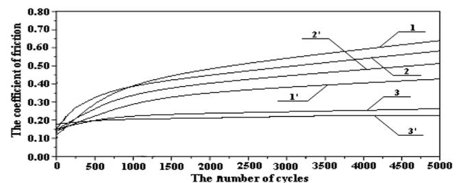
Fig. 5. Dependence of the friction coefficient on the number of cycles (the number without a prime corresponds to the material with a CG structure, the number with a prime corresponds to the material with a UFG structure): 1 - 1' - commercially pure titanium Grade 4; 2 - 2' - commercially pure titanium Grade 4 with IPS coating (TiC); 3 - 3' - commercially pure Grade 4 titanium with a coating obtained by the MAO technology (TiO).
