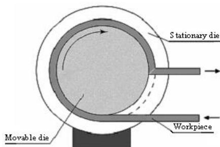
**Fig. 1** Principle of the ECAP-Conform process for producing long-length semi-finished products with ultrafine-grained structure
