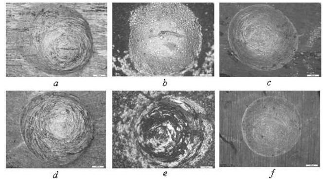
**Fig. 7.** Imprints from the indenter after its impact on CG samples from commercially pure titanium Grade 4 with different surface treatments: a - without coating; b - with TiC coating deposited by ion-plasma spraying; c - with TiO<sub>2</sub> coating, obtained by MAO technology; and on UFG samples: d - without coating; e - coated with TiC; f - with TiO<sub>2</sub> coating, obtained by the MAO technology. (10 times magnification)
