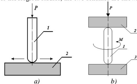
**Fig. 2.** Reciprocal test scheme: a) 1 - spherical indenter; 2 - the test sample; a test scheme for determining the shear strength of adhesion bonds and the molecular component of the friction coefficient: b) 1 - spherical indenter; 2 and 3 are test samples.
