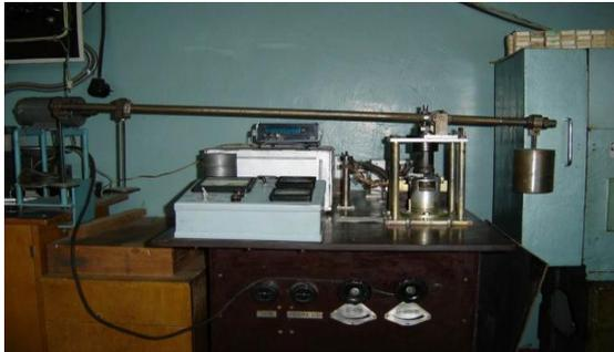
Fig. 4. Equipment for determining the shear strength of adhesion bonds
