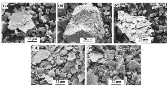
Fig. 2: SEM micrographs of the Al<sub>7</sub>Si powders MA'd for 4 h (a), 8 h (b), 12 h (c), 16 h (d) and 20 h (e).
