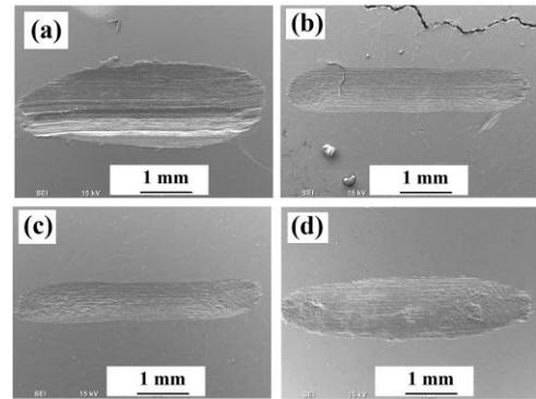
Fig. 6: SEM images of the wear tracks taken from the sintered samples: Al7Si-2LaB<sub>6</sub> (a), Al7Si-2NbB<sub>2</sub> (b), Al7Si-2VB (c), Al7Si-2TiB<sub>2</sub>.
