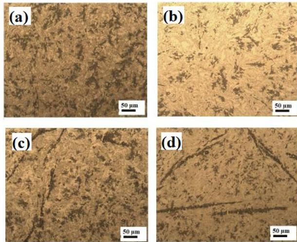
Fig. 5: OM images of the sintered boride reinforced Al7Si samples: Al7Si-2LaB<sub>6</sub> (a), Al7Si-2NbB<sub>2</sub> (b), Al7Si-2VB (c), Al7Si-2TiB<sub>2</sub> (d).
