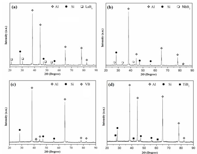
Fig. 3: XRD patterns of the boride reinforced Al<sub>7</sub>Si powders MA'd for 12 h: Al<sub>7</sub>Si-2LaB<sub>6</sub> (a), Al<sub>7</sub>Si-2NbB<sub>2</sub> (b), Al<sub>7</sub>Si-2VB (c), Al<sub>7</sub>Si-2TiB<sub>2</sub> (d).
