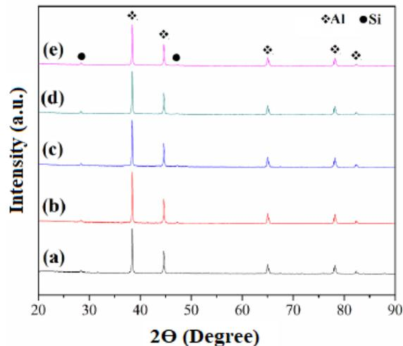
Fig. 1: XRD patterns of the Al<sub>7</sub>Si powders MA'd for 4 h (a), 8 h (b), 12 h (c), 16 h (d) and 20 h (e).
