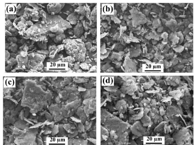
Fig. 4: SEM micrographs the boride reinforced Al<sub>7</sub>Si powders MA'd for 12 h: Al<sub>7</sub>Si-2LaB<sub>6</sub> (a), Al<sub>7</sub>Si-2NbB<sub>2</sub> (b), Al<sub>7</sub>Si-2VB (c), Al<sub>7</sub>Si-2TiB<sub>2</sub>.
