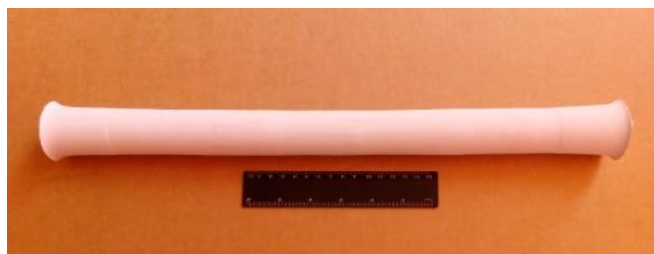
Fig. 4 The appearance of the pressed ceramic insulator based on aluminum oxide
