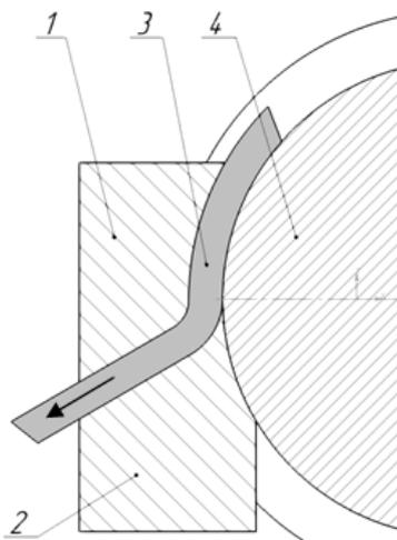
**Figure. 1.** A schematic diagram of the bending of samples due to active friction forces according to the "Conform" scheme in a stationary bending matrix: 1, 2 - two matrix elements for bending; 3 - sample; 4 - drive roller with engraving
