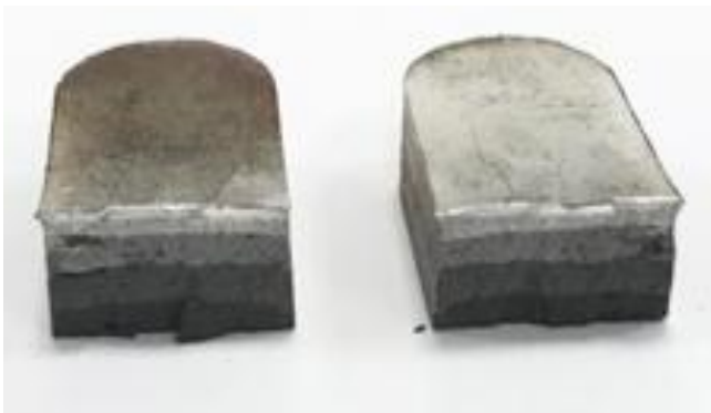
Fig. 2 Image of the FGM after bending test, exposing the 4 levels in its structure.
