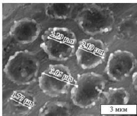
**Fig.1** Microcraters obtained by femtosecond laser titanium irradiation [10]
