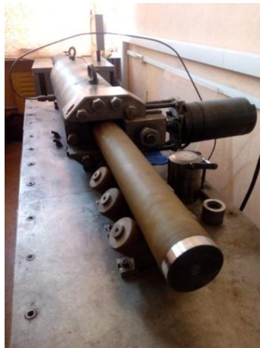
Fig. 1. External view of the isostatic pressing equipment ISPR.1
