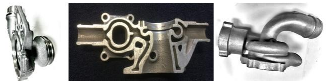
Fig.1 Photos of aluminium parts casted in to 3D-printed sand. The moulds are made up of segments printed in industrial printers.
