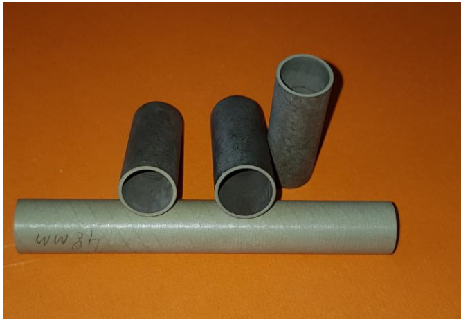
Fig. 4 A view of the blanks of a tubular propelling device for precise movements
