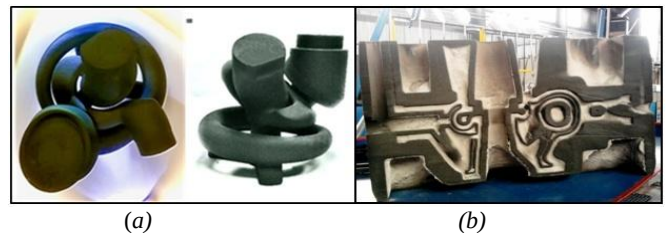
Fig. 2 Photos of 3d-printed sand segments: a) Two views of central-core in 3D-printed sand; b) 3D-printed core "Monobloc" with the highest complexity
